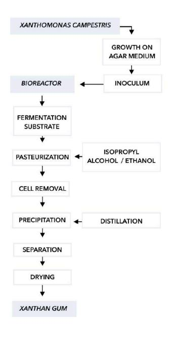
Figure 1: Model of the Xanthan Gum production process.
